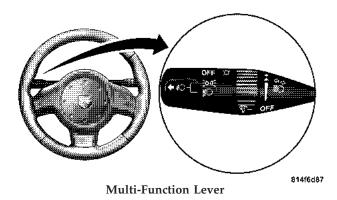
To change the brightness of the instrument panel lights, rotate the center portion of the Multi-Function Control Lever up or down.
